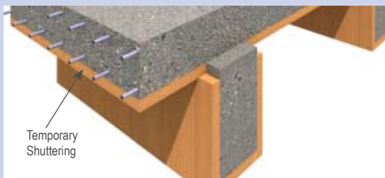
Temporary Shuttering removed after slab sets
